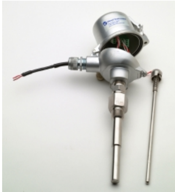
Photo D – RTD Assembly with TEDS Option
